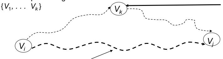
Shortest Path using intermediate vertices {  $V_{1}, ..., V_{k-1}$  }
